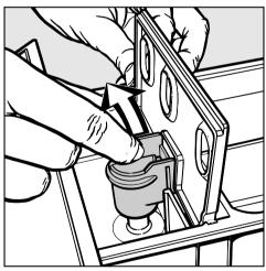
■ Remove the suction tube from compartment , wash under running warm water and replace.
